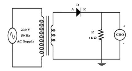
HALF WAVE RECTIFIER (WITH FILTER):
